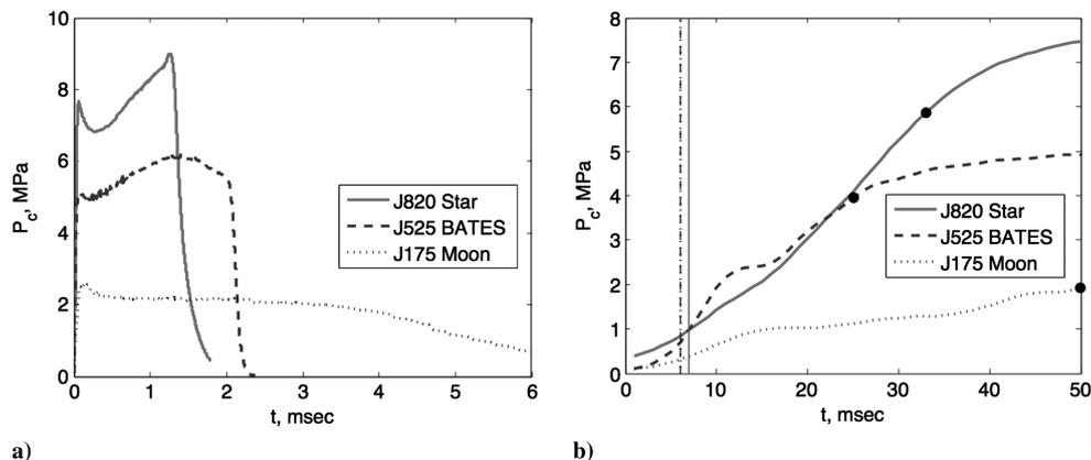
Fig. 6 Typical a) overall and b) startup pressure traces, with  $t_{id}$  and rise time noted.
