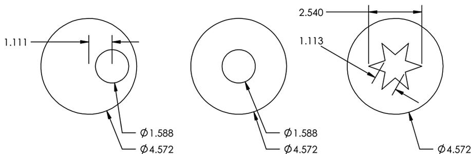
**Fig. 1 End-on views of moon, BATES, and star geometries (dimensions in cm).**
