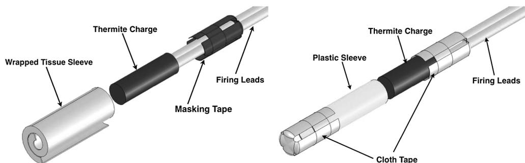
Fig. 4 Paper (left) and plastic (right) containment methods for thermite charges.
