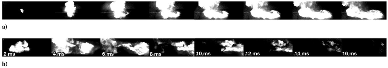
Fig. 2 Time-synchronized images of a) paper-contained and b) plastic-contained igniters.
