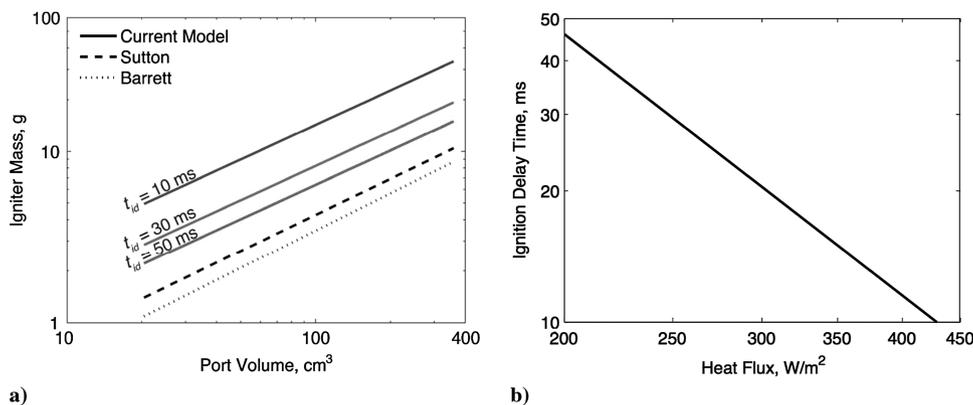
Fig. 3 Predictions for a) igniter size vs port volume, and b)  $t_{\text{id}}$  vs heat flux.
