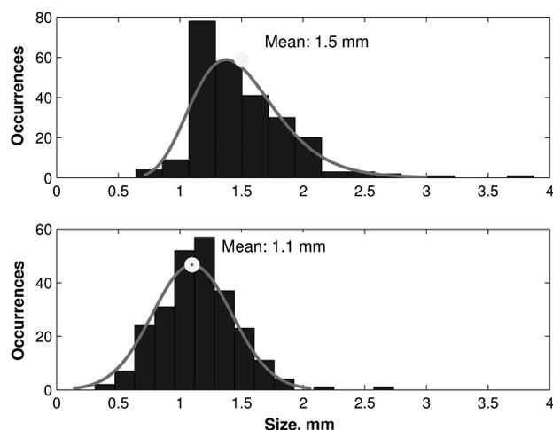
Fig. 5 Condensed phase product size distributions for paper (top) and plastic (bottom) containment techniques.
