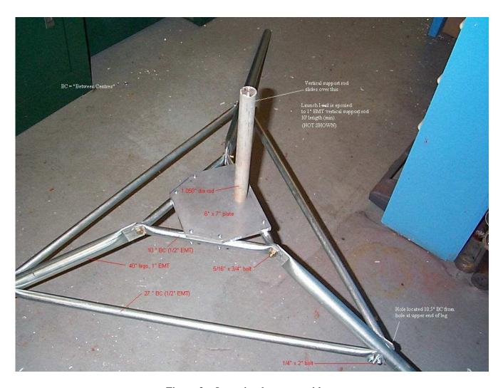
Figure 2 – Launcher base assembly
