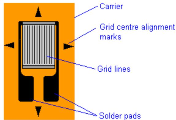
Figure 1 – Strain gage
