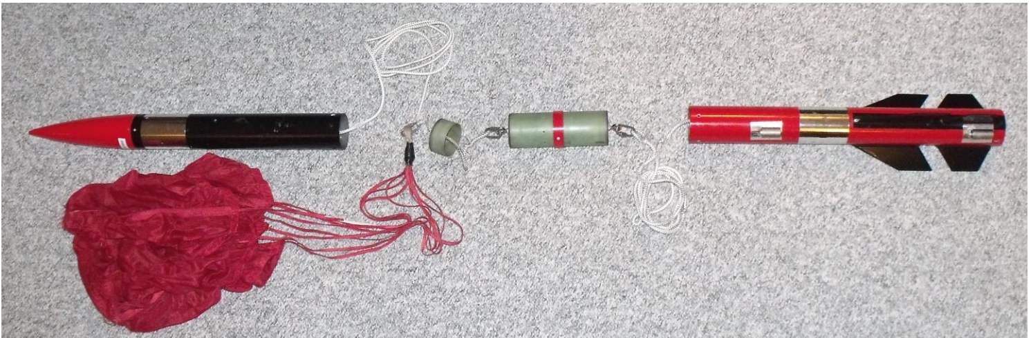
Figure 2 – DS Rocket dis-assembled to show deployment components
